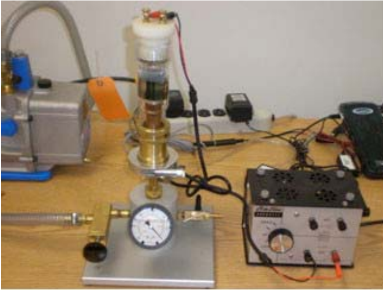
Figure 6. VPAL-A configured for metal evaporation. Photo courtesy of Robert Decker.
